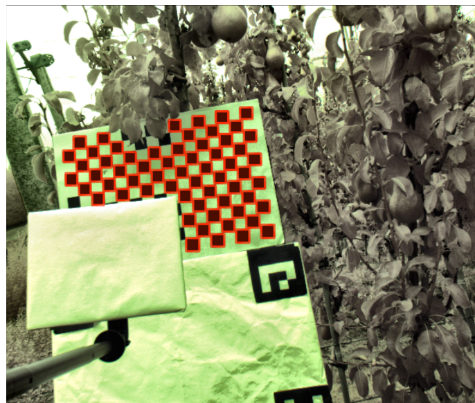
Fig. 7: The average size of the black squares is used to estimate the conversion from uncalibrated units to meters.
